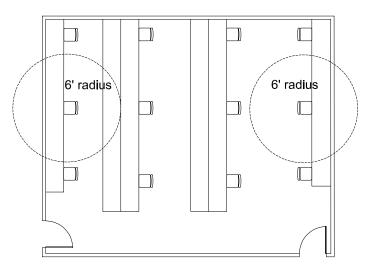
CLASSROOM SOCIAL DISTANCING PLANS COMPUTER LAB PROTOTYPE A 05 JUNE 2020 COMPUTER LAB PROTOTYPE B 46 SEATS AT 36" SP 964 SF 21 SF/ST
